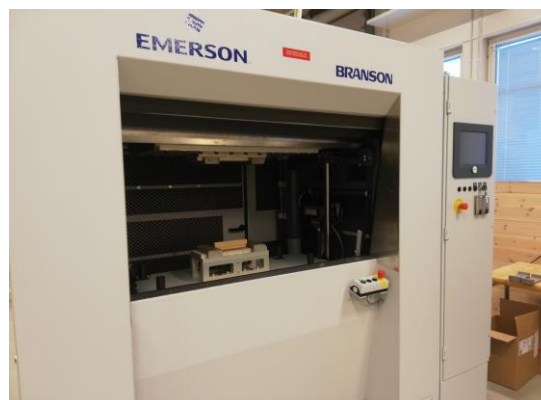
Figure 1. Linear vibration-welding machine
