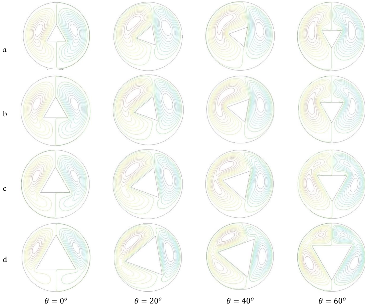
Figure 6. Streamlines for (a) RR = 3.0, (b) RR = 2.5, (c) RR = 2, and (d) RR = 1.5 at different inclination angles and Ra = 10^5 .
