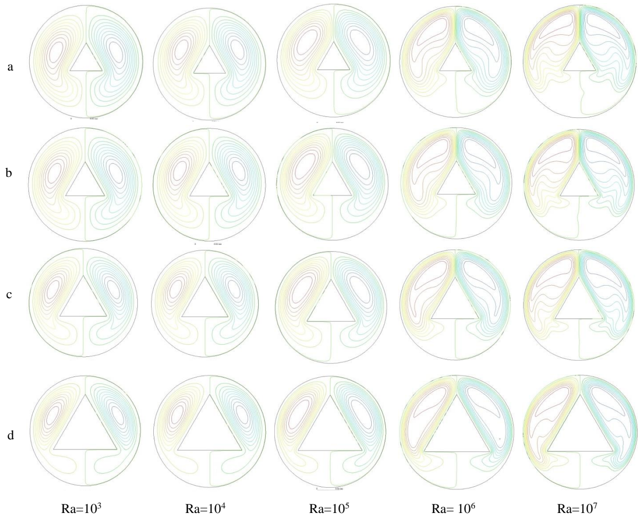
Figure 5. Streamlines for (a) RR = 3.0, (b) RR = 2.5, (c) RR = 2, and (d) RR = 1.5 at \theta = 0^\circ and various Ra.
