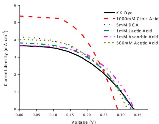
**Fig. 4.** Current – voltage behaviour of the DSSCs fabricated using *Melastoma malabathricum* L. (KK) dye treated with different acids.
