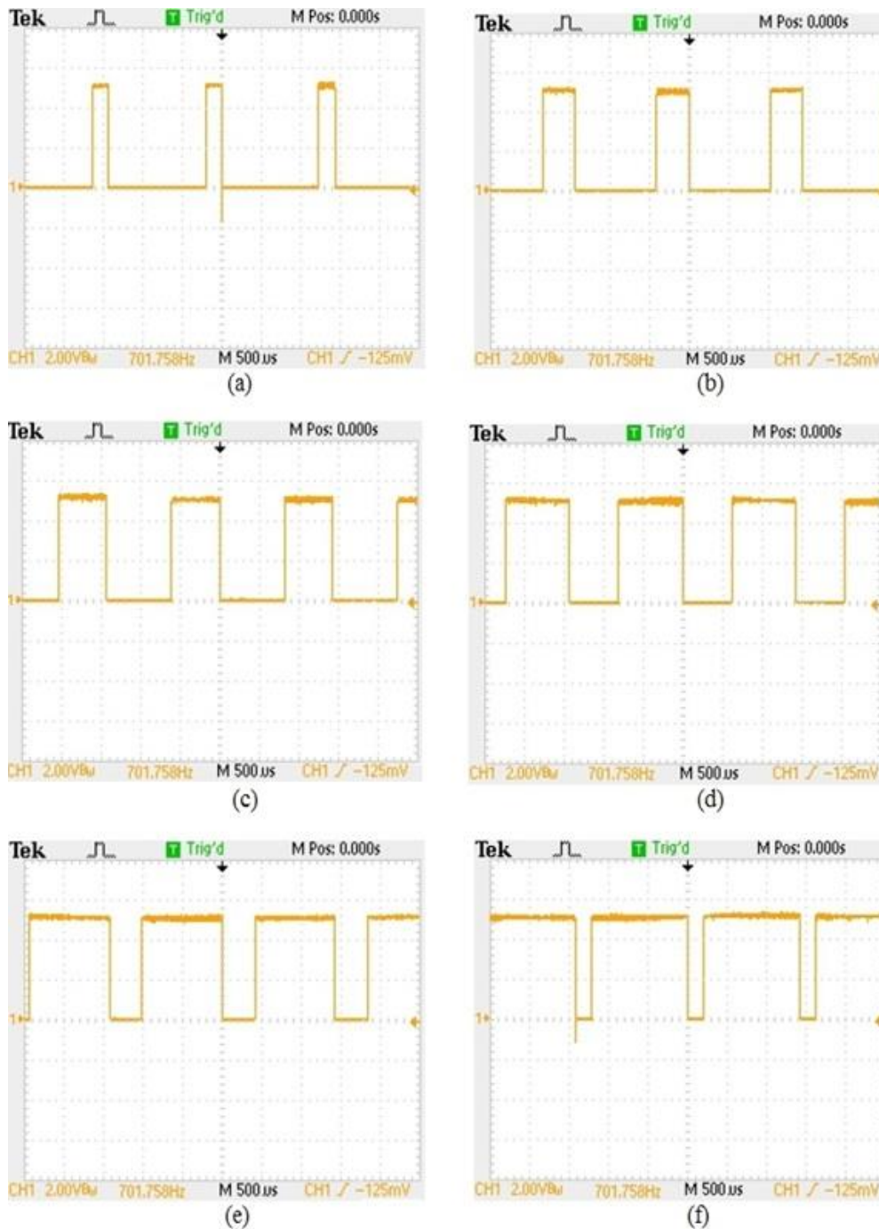
Fig. 5. PWM signal for LED dimming for 6 different lighting levels, PWM generated for (a) control signal 1, (b) control signal 2, (c) control signal 3, (d) control signal 4, (e) control signal 5, (f) control signal 6
