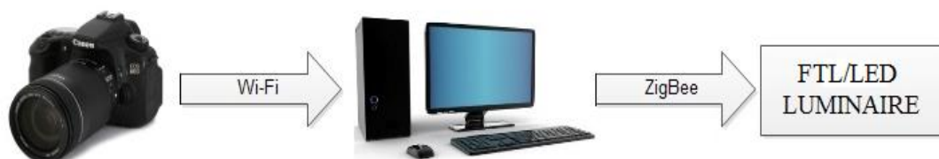
Fig. 1. HDRI system for automatic lighting control
