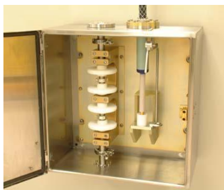
Fig. 13. A co-field treatment chamber designed by Kempkes et al. [15].
