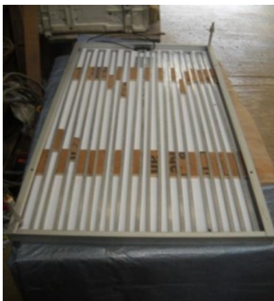
Figure 2. Installation of oscillatory flow heat exchanger at bottom side of PV module
