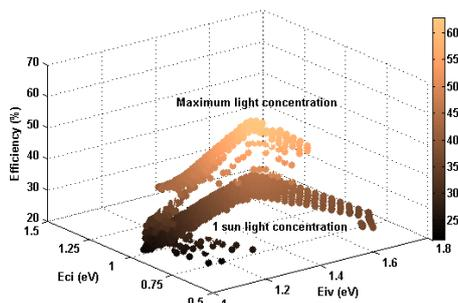
**Fig. 9.** Detailed balance efficiency of QD solar cell one- IB varies with  $E_{iv}$  and  $E_{ci}$  at blackbody spectrum under 1 sun and maximum light concentrations
