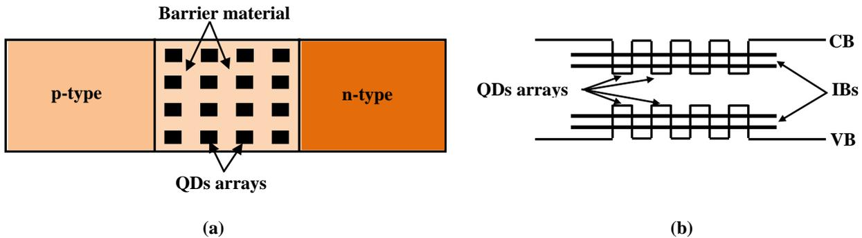
**Fig. 1.** (a) Schematic diagram of the QDs inside a bulk semiconductor of larger bandgap (b) Intermediate energy bands of an array of QDs
