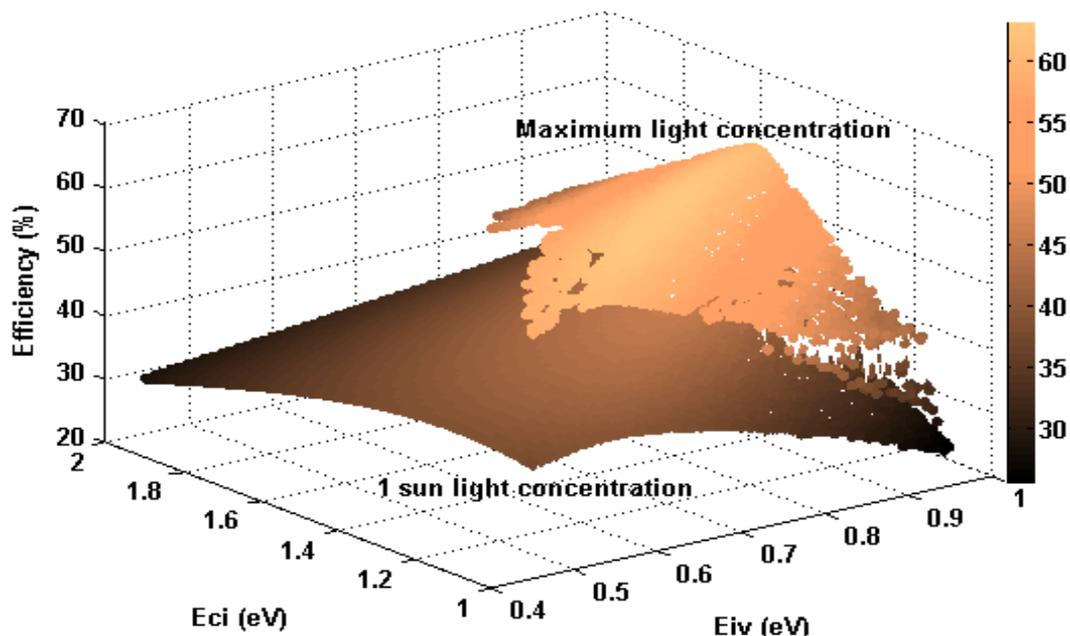
**Fig. 3.** Detailed balance efficiency of one-IBSC varies with the place of IB between the CB and VB at blackbody spectrum under 1 sun, and maximum light concentrations
