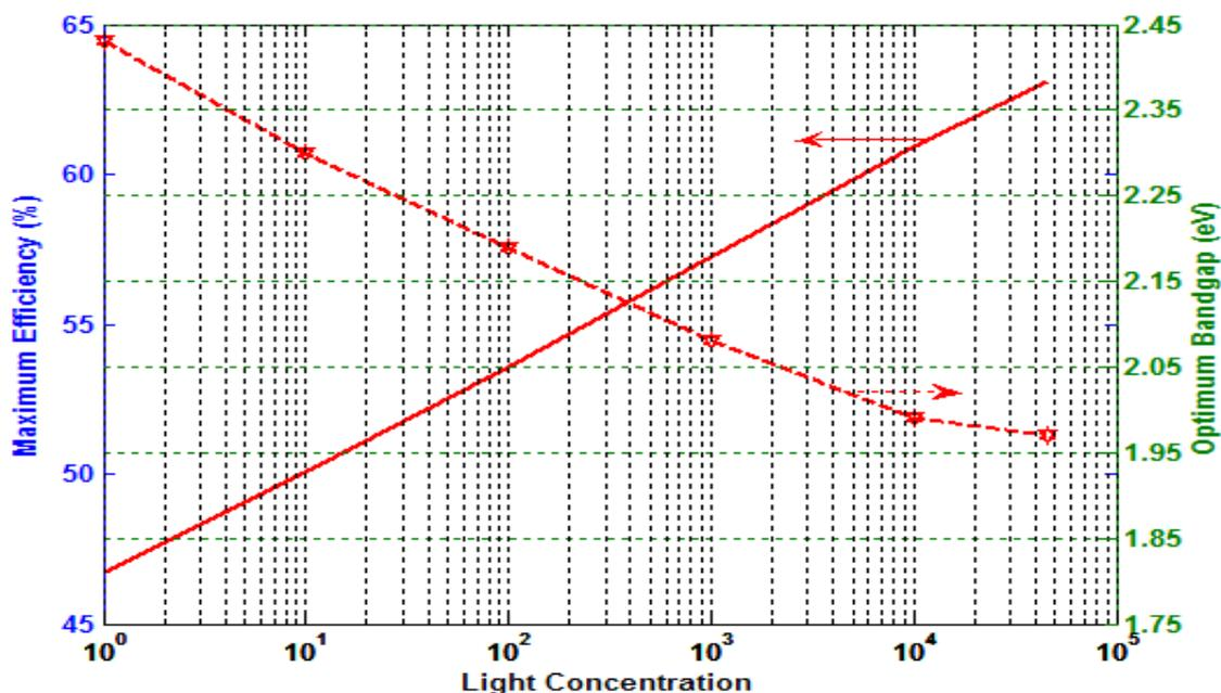
Fig. 4. Maximum efficiency and optimum bandgap energy,
