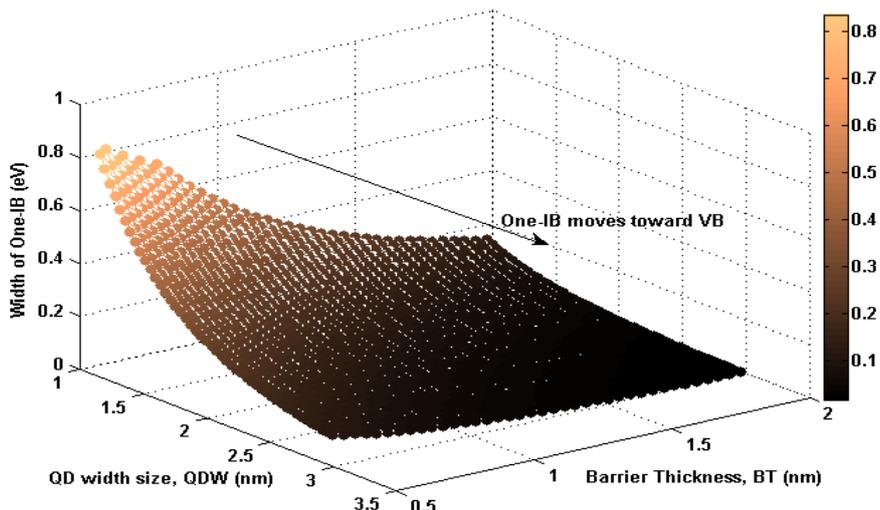
**Fig. 5.** The relation between width of one-IB energy and each of QDW and BT
