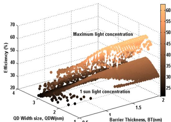
**Fig. 8.** Detailed balance efficiency of QD solar cell one- IB varies with QDW and BT at blackbody spectrum under 1 sun and maximum light 1090
