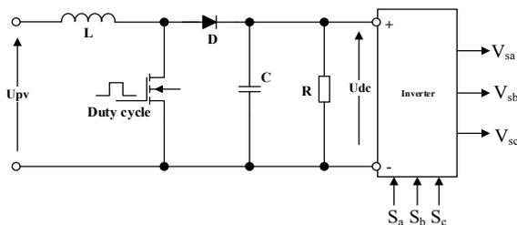
**Fig. 5.** DC-DC converter circuit schema
