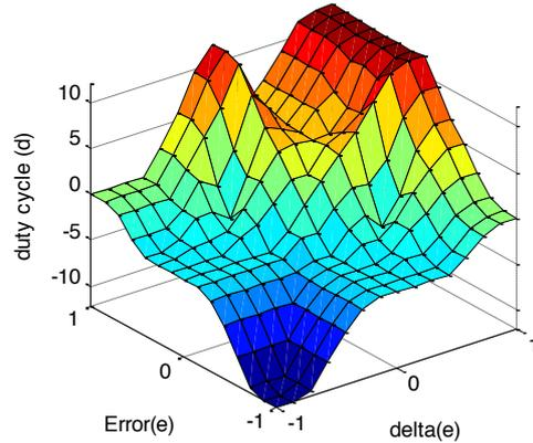
Fig. 9. Surface of fuzzy logic controller
