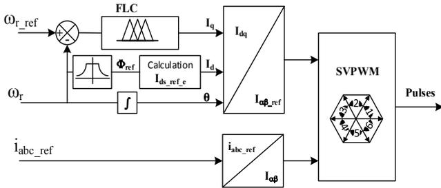
Fig. 10. Speed control of PMSM
