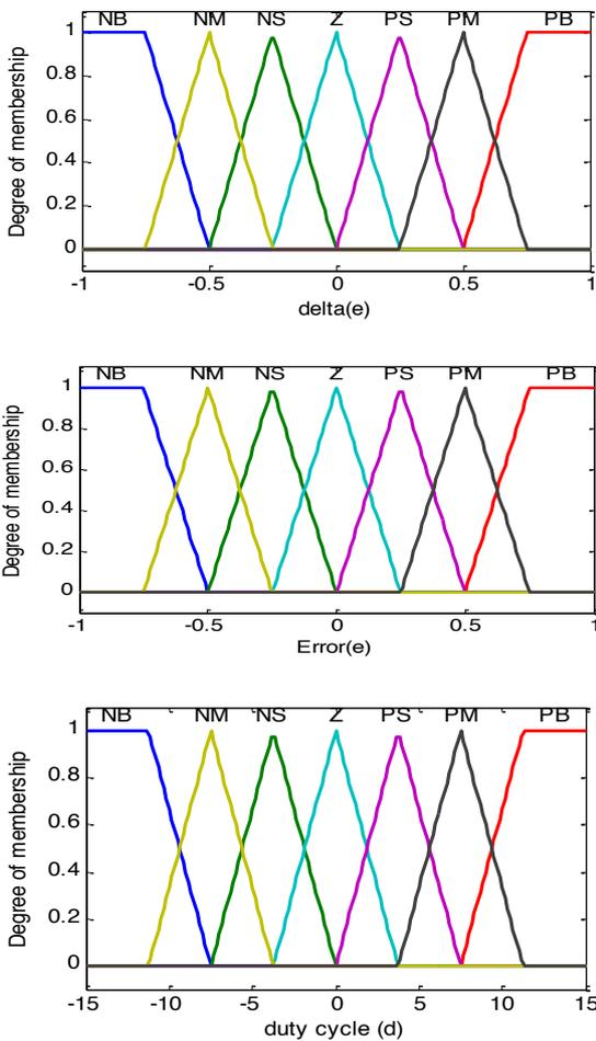
Fig. 8. Rules of fuzzy logic controller
