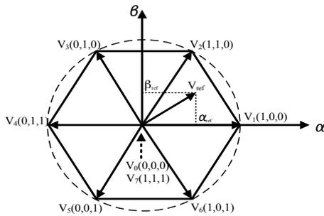
Fig. 6. Voltages space vector diagram for the two-level inverter
