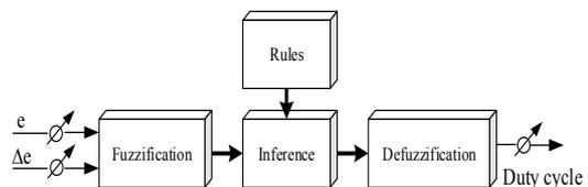
Fig. 7. Structure of fuzzy logic controller
