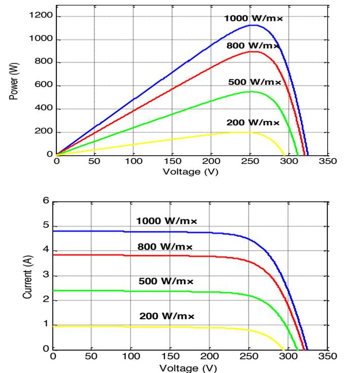
Fig. 3. Power and current characteristics for different solar radiation
