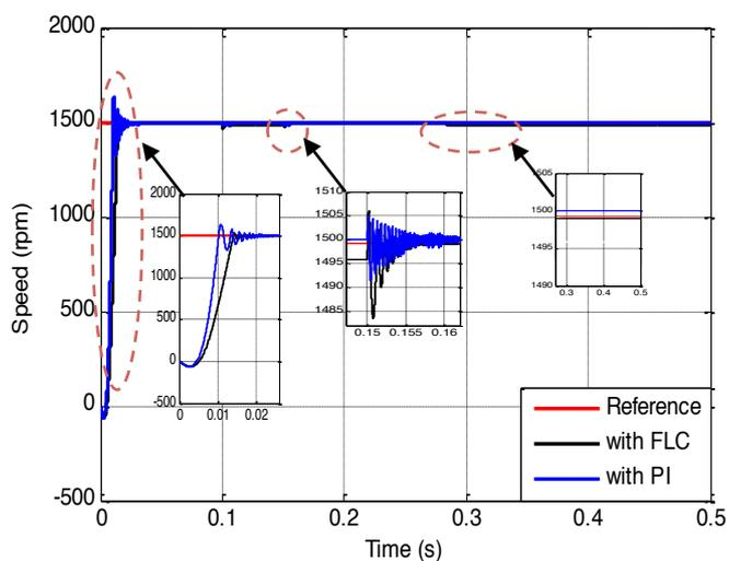
**Fig. 15.** Speed control of PMSM.
