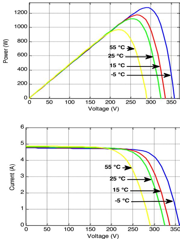
**Fig. 4.** Power and current characteristics for different temperature
