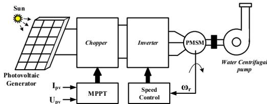
Fig. 1. Synoptic bloc of photovoltaic water pumping
