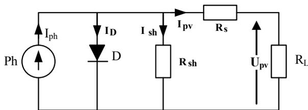
Fig. 2. Equivalent circuit for the photovoltaic model
