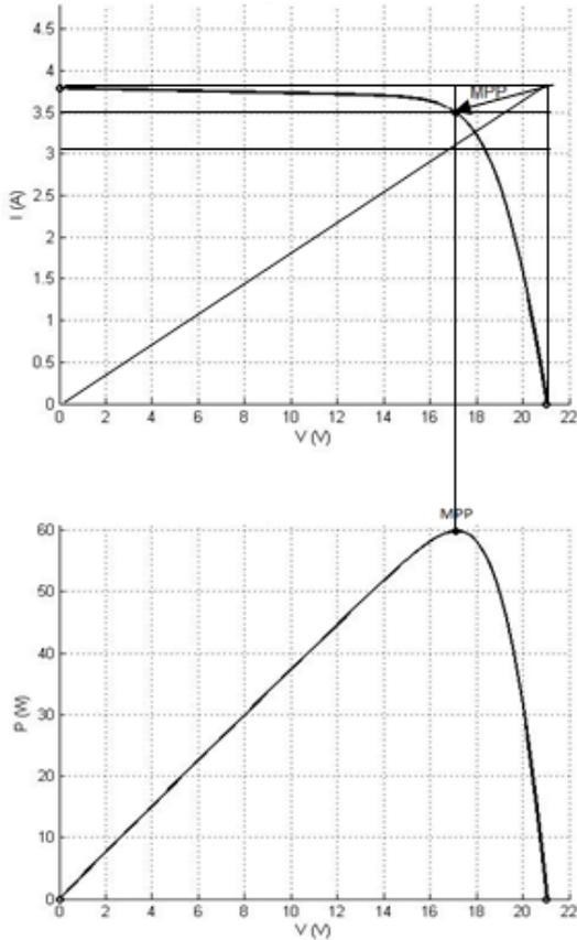
Fig. 5. Mechanism of maximum power point (MPP) angle method for MPPT
