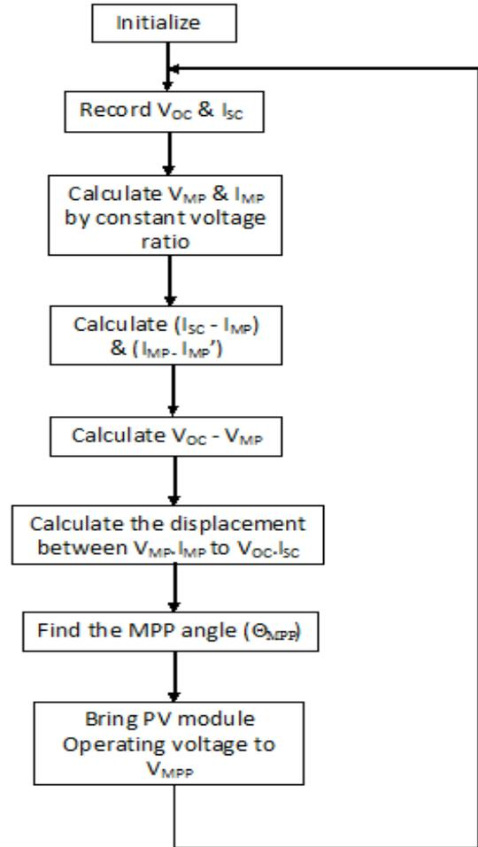
Fig. 7 Maximum Power Angle (MPA) algorithm
