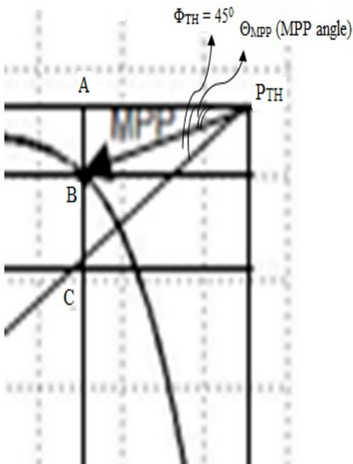
Fig. 6. Parameters of MPA method for MPPT
