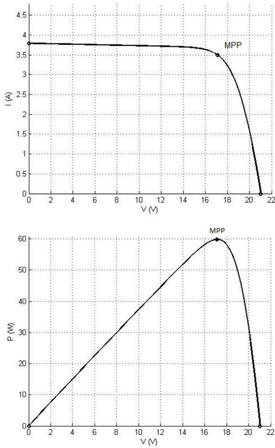
Fig. 4. Simulated I-V and P-V Characteristic Curves
