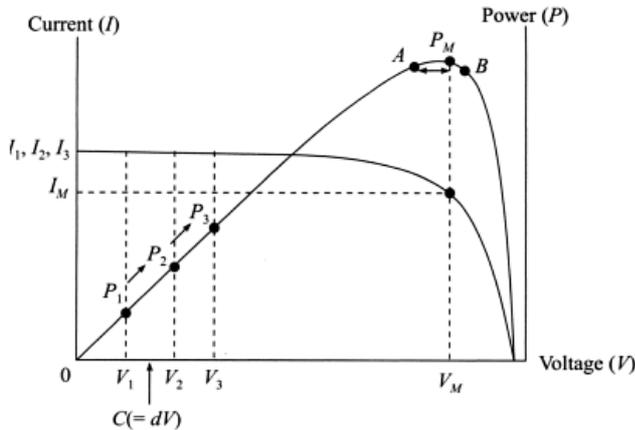
Fig. 1. Perturb and Observe (P&O) Technique for MPPT
