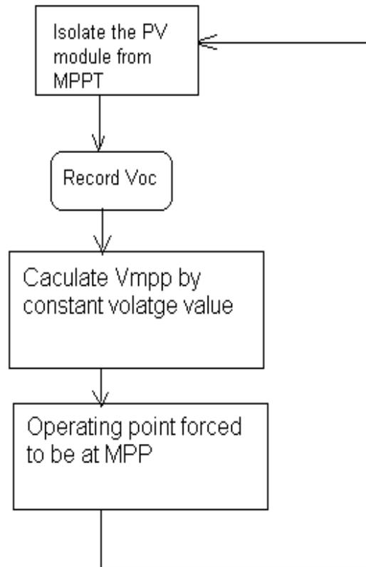
Fig. 3. Structure of Constant Voltage method
