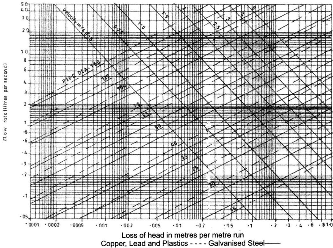
Fig. 5. Pipe Sizing Graph
