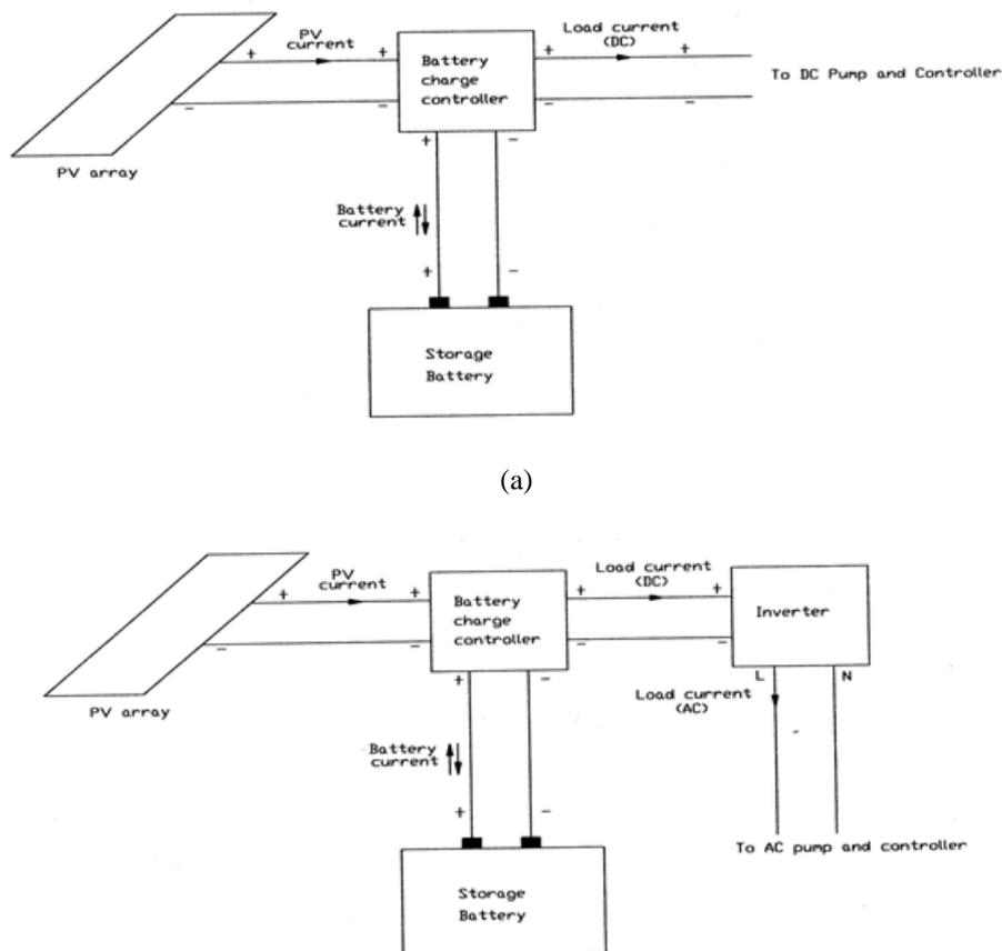
**Fig. 4.** a: PV System Incorporating a Battery and Charge Controller to Produce DC, b: PV System Incorporating an Inverter to Produce AC
