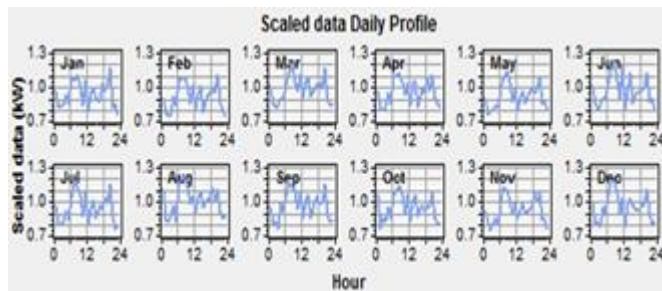
Fig.4. Hourly load profile of the telecom tower site
