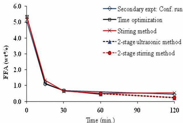
Fig. 3. FFA reduction with different reaction time and two-stage esterification
