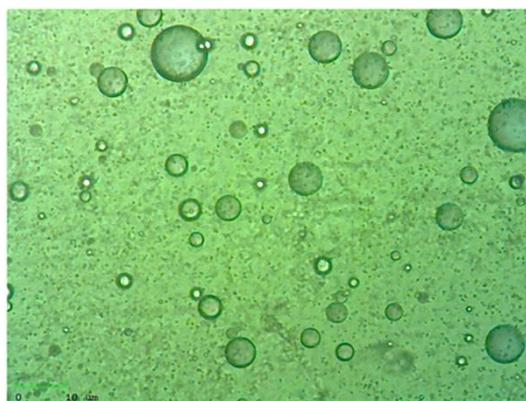
**Fig. 5.** The reaction mixture obtained by stirring method after 1 h reaction time, 100X magnification.
