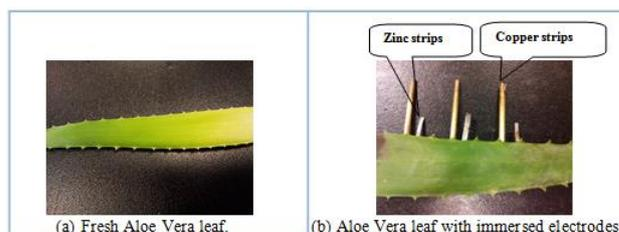
**Fig. 2.** Photos showing without electrodes immersed (fresh Aloe Vera) and with electrodes (copper and zinc) immersed.
