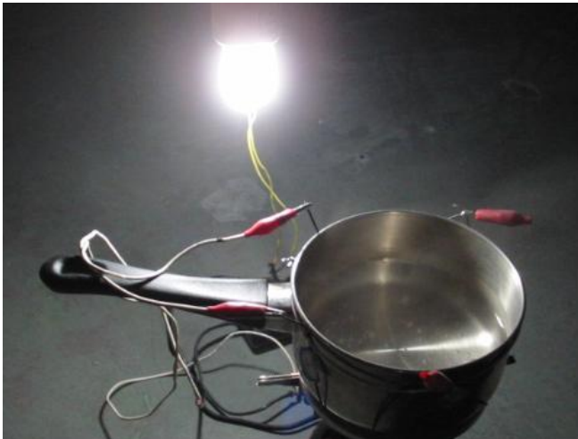
Fig.2. Hot water can be used to turn on the Lights with the Thermoelektrik Module(Source: http://www.tegpower.com )
