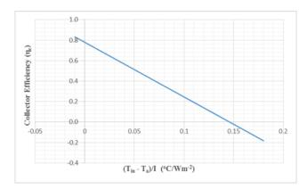
Fig. 5. Performance characteristics curve of a flat-plate collector at  $T_a = 25.7^{\circ}C$
