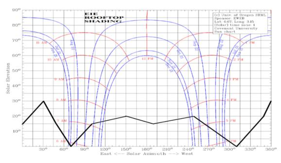
Fig. 4. Shading plots for a test location at the rooftop of the EIE office building
