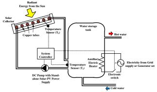
Fig. 1. The microcontroller-based ASWHS schematic diagram
