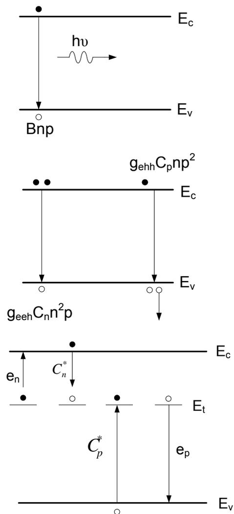
**Fig. 1** Radiative, Auger and SRH recombination process, respectively.
