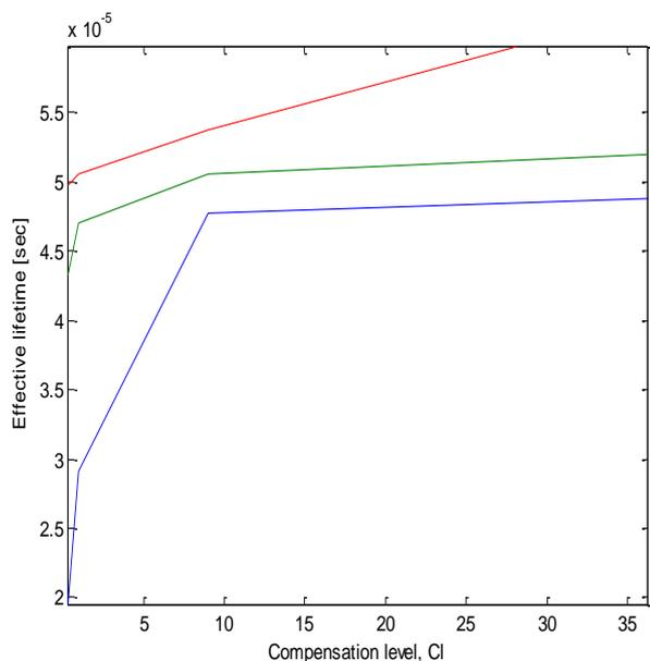
**Fig.6.** Effective lifetime of minority carrier in compensated p-Si solar cell.
