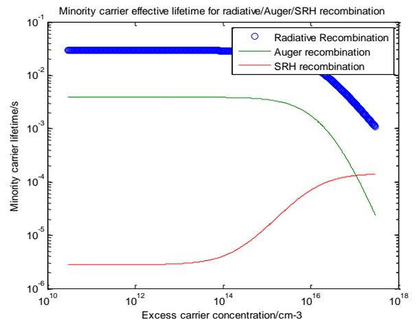
**Fig.2.** Bulk recombinations lifetime (SRH recombination, radiative recombination and free particle Auger recombination.) for noncompensated p-Si solar cell [11].
