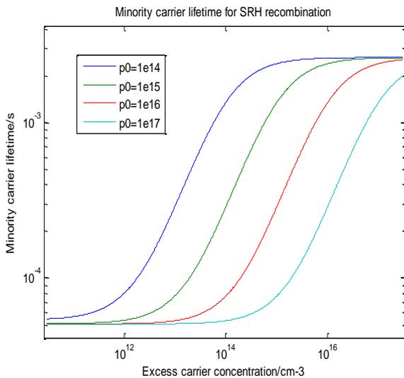
**Fig.3.** Injection dependent SRH lifetime for four different values of  $p_0$  for compensated p-Si solar cell.
