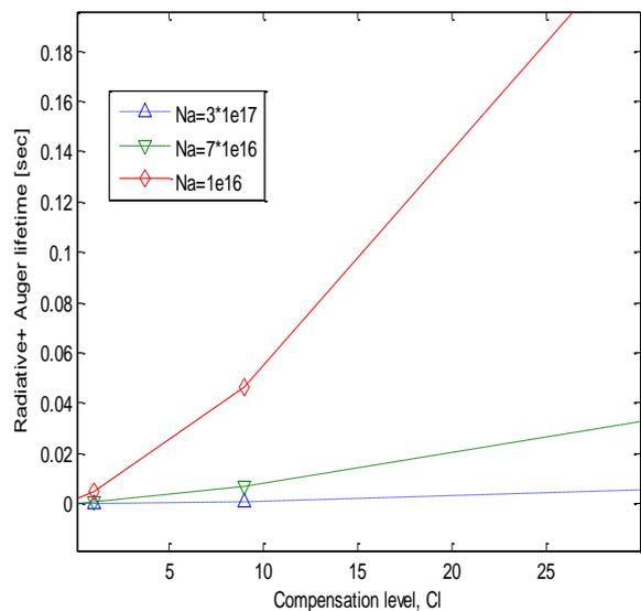
**Fig.5.** Intrinsic lifetime of compensated p-Si solar cell.
