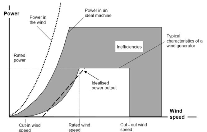
**Fig. 8.** A wind turbine characteristic
