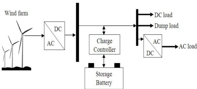
**Fig. 7.** Typical wind power system
