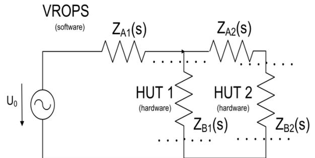
**Fig. 6.** Impedance network as an example for MIMO PHIL
