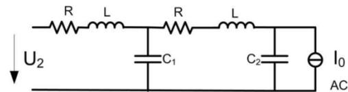
Fig. 10. Modelling of the PV inverter for stability determination purpose
