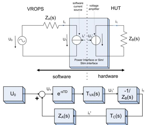
**Fig. 3.** Basic PHIL setup with PI and ITM IA and the corresponding signal flow diagram
