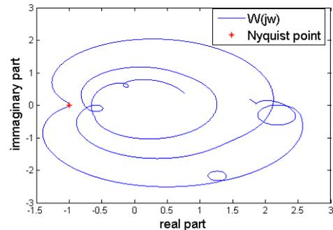
Fig. 12. Nyquist plot for PCD interface (common resistor R=0.5Ohm)
