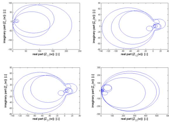
**Fig. 8.** Distribution network with two PV inverters feeding in considered in the case study (left), Locus plot of the entries of the impedance matrix of the network (right)
