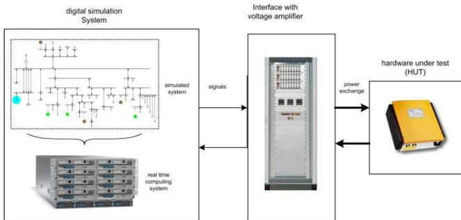
**Fig. 1.** Typical PHIL configuration (SISO)
