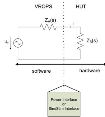
**Fig. 2.** Basic circuit for introducing the idea of the PHIL simulation
