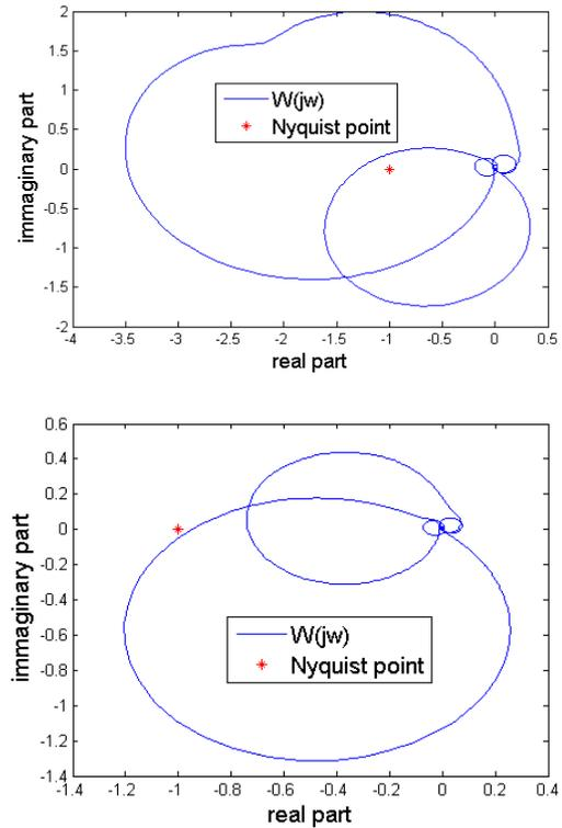
Fig. 11. Nyquist plot for ITM IA without and with additional hardware inductance
