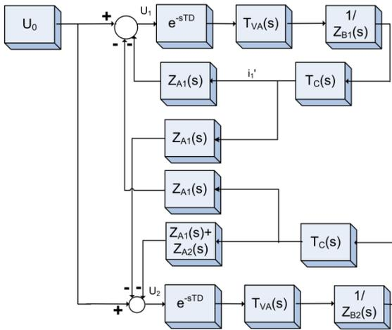
**Fig. 7.** Signal flow diagramm of the MIMO PHIL example in Fig. 6
