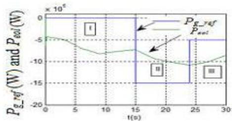
Fig. 8. Grid reference and DFIG active powers
