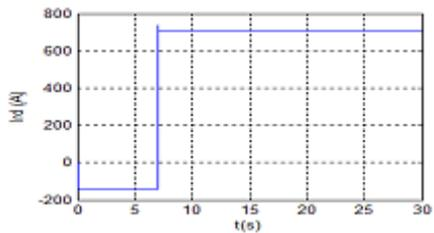
Fig. 6. Direct rotor current component
