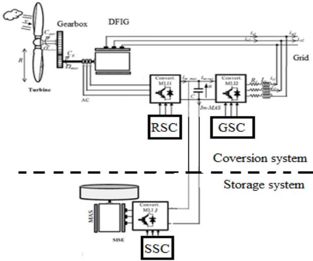
**Fig. 1.** Wind energy conversion and storage system (WECSS)
