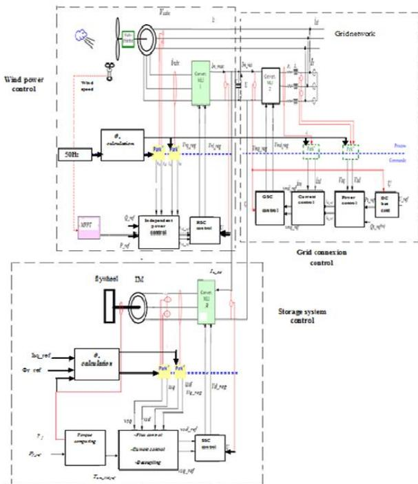
Fig. 3. A completed conversion system control schematic.
