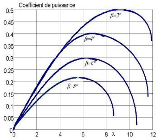
**Fig. 2.** Power coefficient [12]
