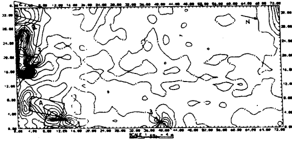
Şekil 6: 0.25 devir/m kesme frekanslı alçak geçişli filtre haritası. Figure 6: The map of the low pass filter with 0.25 cycle/m cutting frequency.
