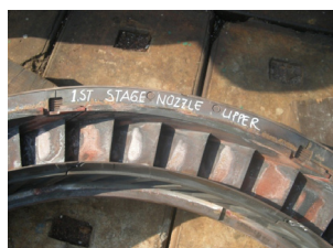
Figure 13. Visual inspection of 1st stage turbine nozzle (erosion material) after operated with B5
