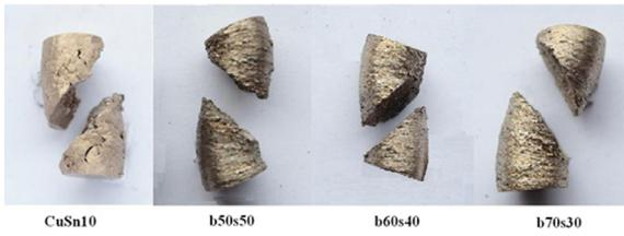
**Figure 6.** Fracture morphologies of the MMC materials
