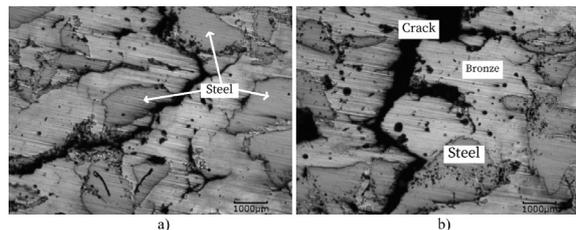
**Figure 8.** Microstructure of the b50s50 material (50X)
