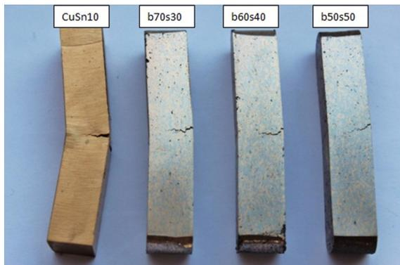
**Figure 10.** Crack formation in the bending specimens
