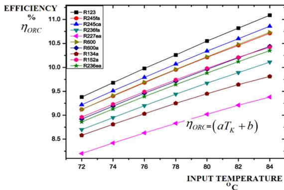
Figure 3. ORC Efficiencies for different working Fluids [8]
