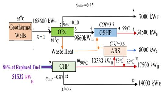
**Figure 13.** Conceptual System for the new settlement (X=1)
