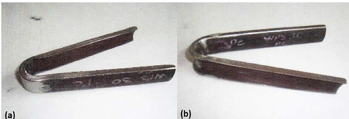
Figure 9. Bending test sample type photos; (a) Face bend, (b) Root bend
