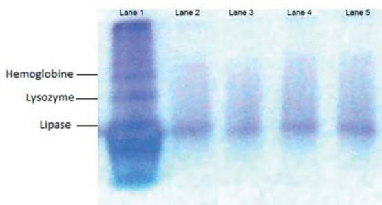
**Figure 12.** SDS-PAGE image for lipase enzyme desorbed from *Candida cylindracea*. Lane 1: Marker (Lipase, Lysozyme, Hemoglobine) Lane 2: Lipase marker, Lane 3: Initial lipase solution [(Before adsorption for Cu nanoparticle embedded poly(HEMA-MATrp) cryogels], Lane 4: Final lipase solution [(After adsorption for Cu nanoparticle embedded poly(HEMA-MATrp) cryogels], Lane 5: Desorbed sample [(After desorption from Cu nanoparticle embedded poly(HEMA-MATrp) cryogels).
