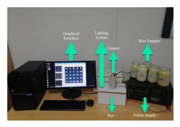
Figure 2- Mechanism used to obtain images
