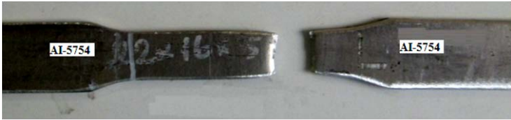
Figure 3. Tensile test fracture surfaces Al 5754 base material
