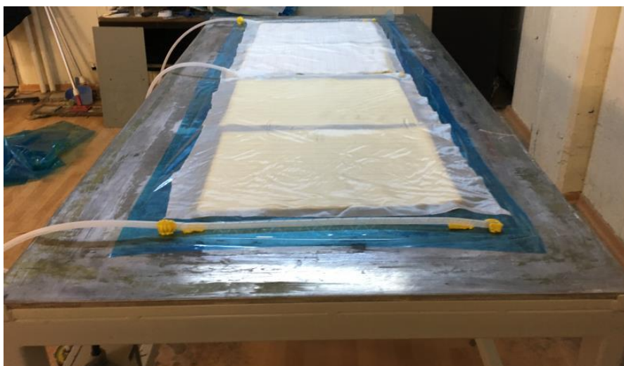
Figure 2. Production of glass fibre/epoxy composite plates by VARIM
