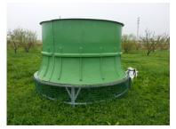
Figure 4. Overview of Upward-Blowing Wind Machine
