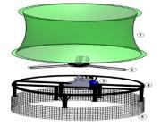
Figure 5. Parts of upward-blowing wind machine are; 1. Fan Chimney, 2. Fan Kit, 3. Engine, 4. Construction 5. Protection cage.
