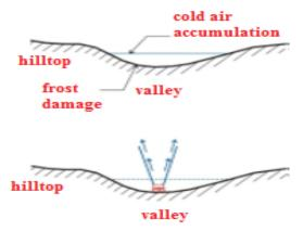
Figure 1. Selective Cold Air Drainage
