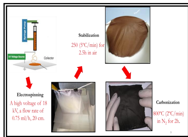
Figure 1 Schematic diagram of carbon nanofiber (CNF) formation.
