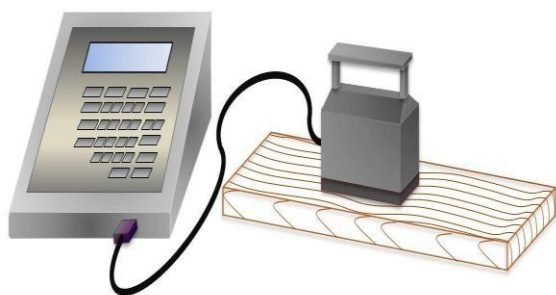
Fig. 1. Test setup of thermal conductivity measurements
