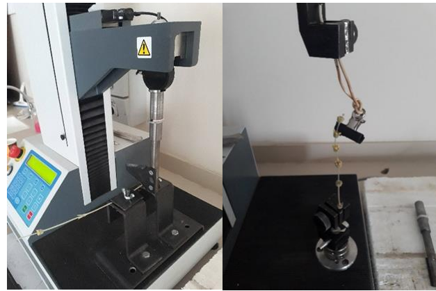
Figure 3. Stalk cutting and flower rupture tests.
