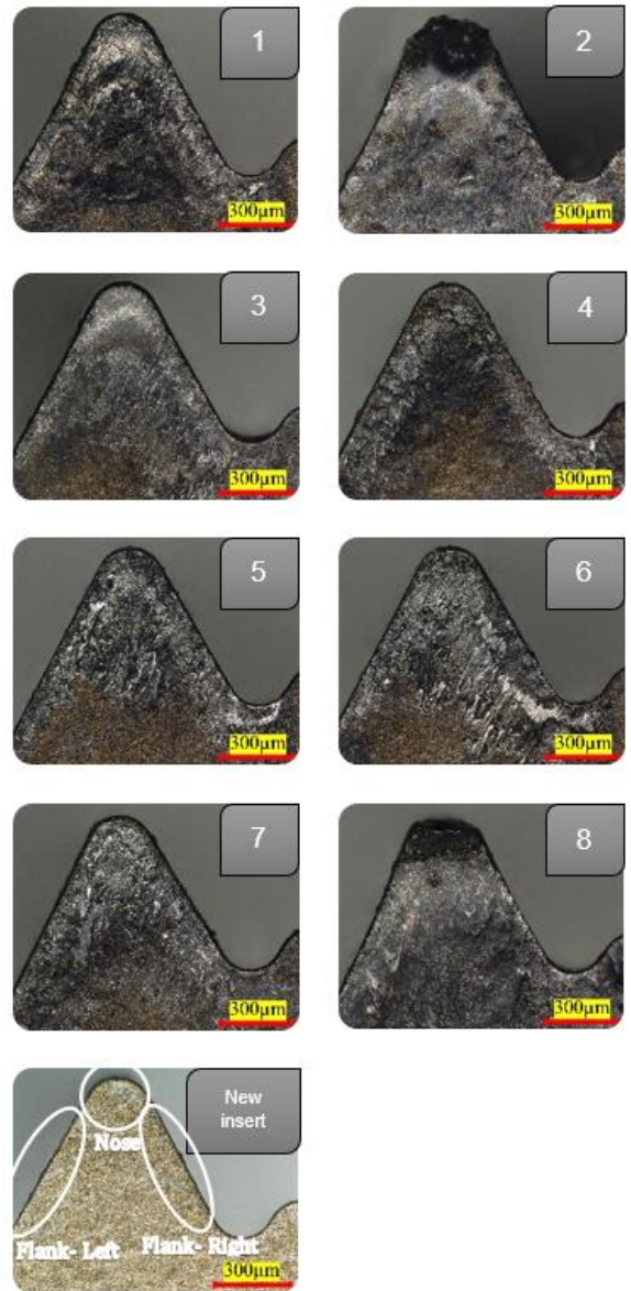
Figure 2. The wear images of the threading insert
