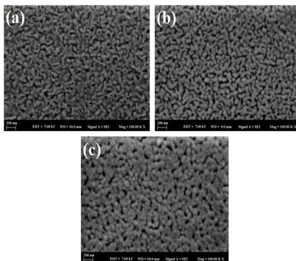
Figure 3. SEM images of (a) pure ZnO, (b) 1% and (c) 50% Cu doped ZnO nanostructure thin films
