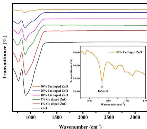
**Figure 5.** FTIR spectra of pure ZnO and ZnO nanostructure thin films with different concentrations (1-50%) of Cu
