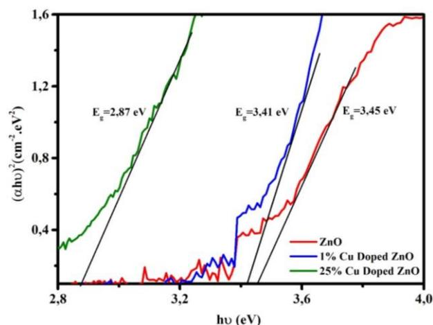
**Figure 7.** Tauc's plot evaluated from UV-Vis absorption spectrum for pure ZnO, 1% and 25% Cu doped ZnO nanostructure thin films
