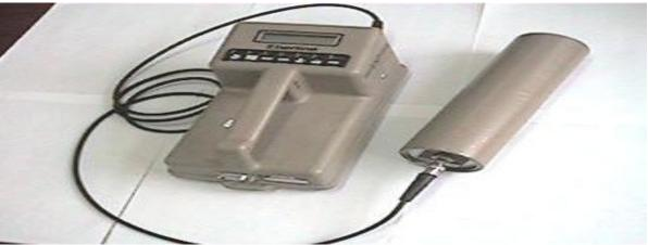
Figure 1: ESP-2 Rate meter and SPA-6 scintillation detector, Eberline (18).
