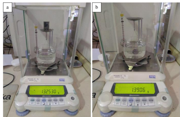
Figure 3. Weighing the specimens in air (a) and water (b)
