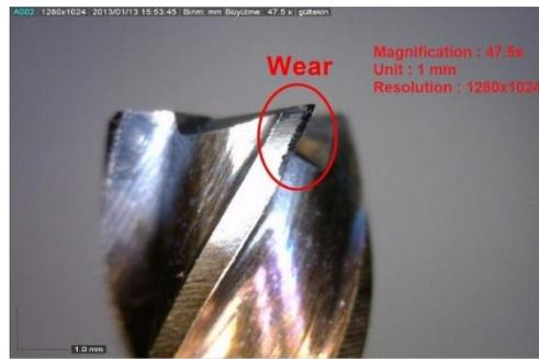
**Figure 5.** Example of a worn end mill (Magnification: 47.5x)
