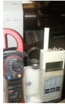
Figure A. Measurement of current value and sound intensity values in the experimental setup
