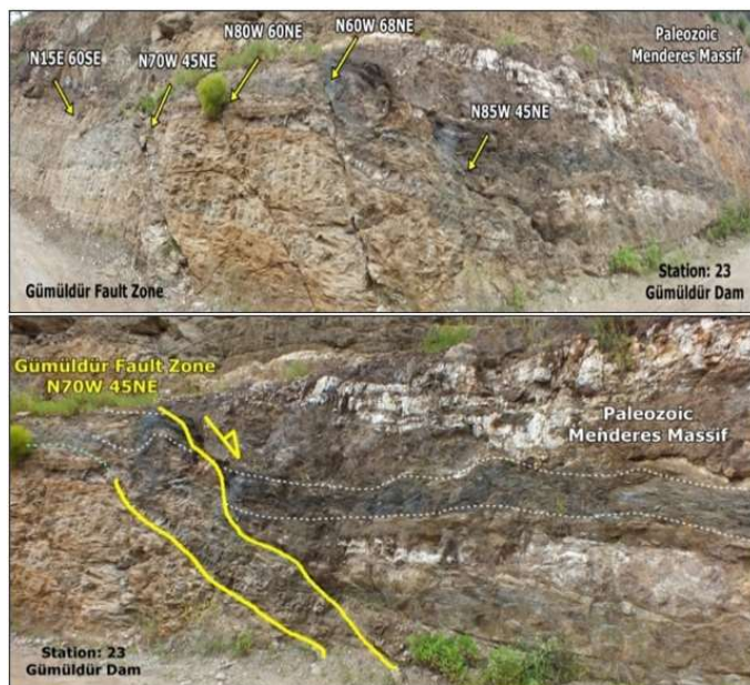
Fig. 8. A view from the faulting of the Gümüldür Fault Zone cutting the Menderes Metamorphics (X: 501098, Y: 4215980)
