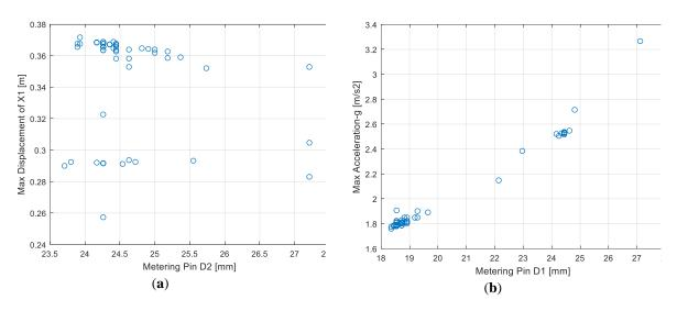
Figure 5. (a) Displacement of aircraft mass vs. D2; (b) Vertical acceleration vs. D1.
