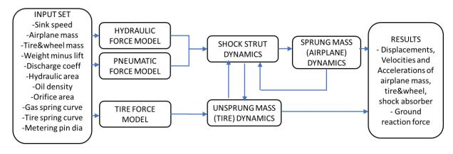
Figure 2. Flowchart of landing gear simulation (adopted from [3]).
