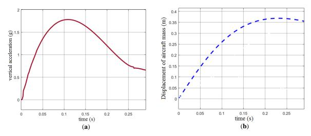
Figure 9. Optimized geometry (a) vertical acceleration (g) vs time (s); (b) displacement of aircraft mass (m) vs time (s)
