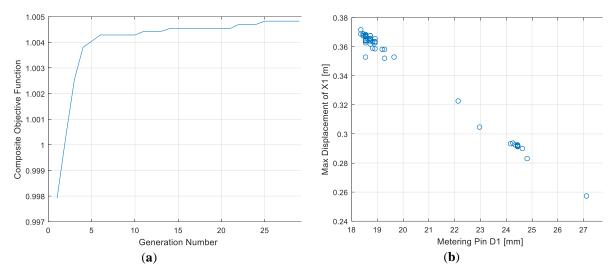
Figure 4. (a) Objective function vs. generations (iterations); (b) Displacement of aircraft mass vs. D1.
