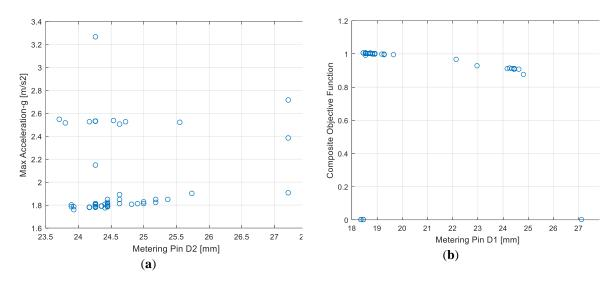
Figure 6. (a) Vertical acceleration vs. D2; (b) Objective function vs. D1.
