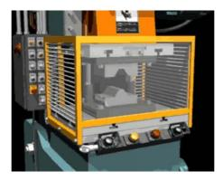
Figure 1. Power press with a fixed barrier guard [13]
