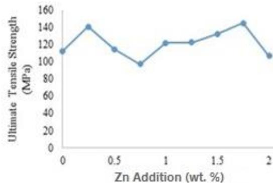
**Figure 4.** Effect of zinc addition on tensile strength of specimens.
