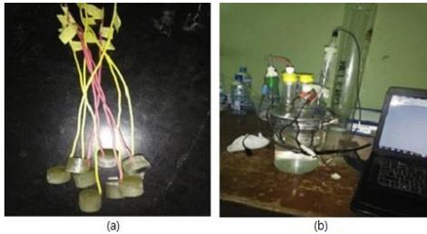
**Figure 2.** (a) Specimens for corrosion test (b) Potentiodynamic polarisation technique setup.
