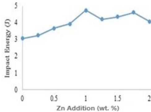
**Figure 6.** Effect of zinc addition on impact energy of specimens.
