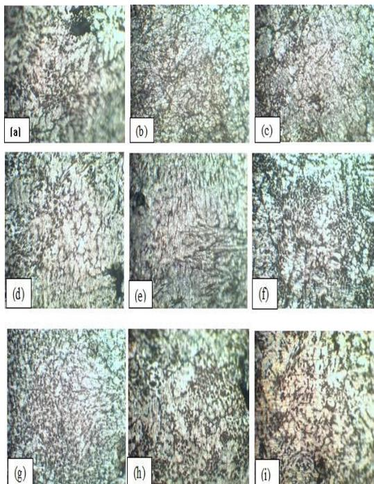
**Figure 7.** Optical micrographs of specimens at varied weight percent (wt. %) of zinc reinforcement (a) 0 (b) 0.25 (c) 0.5 (d) 0.75 (e) 1 (f) 1.25 (g) 1.5 (h) 1.75 and (i) 2 x100.
