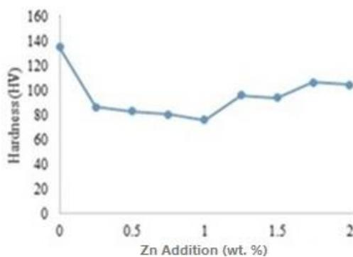
**Figure 3.** Effect of zinc addition on hardness of specimens.
