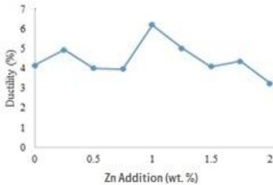
**Figure 5.** Effect of zinc addition on ductility of specimens.
