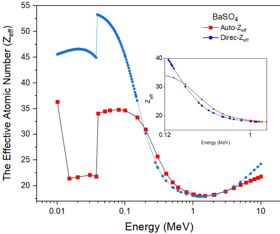
**Figure 2.** The Effective Number ( $Z_{\text{eff}}$ ) comparison of  $\text{BaSO}_4$
