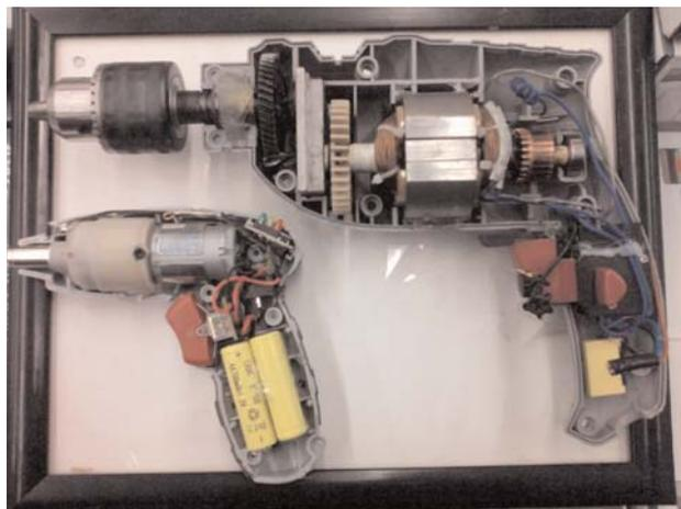
**Fig. 1.** Inner parts of electric drills. [Color figure can be viewed in the online issue, which is available at [www.aott.org.tr](http://www.aott.org.tr)]
