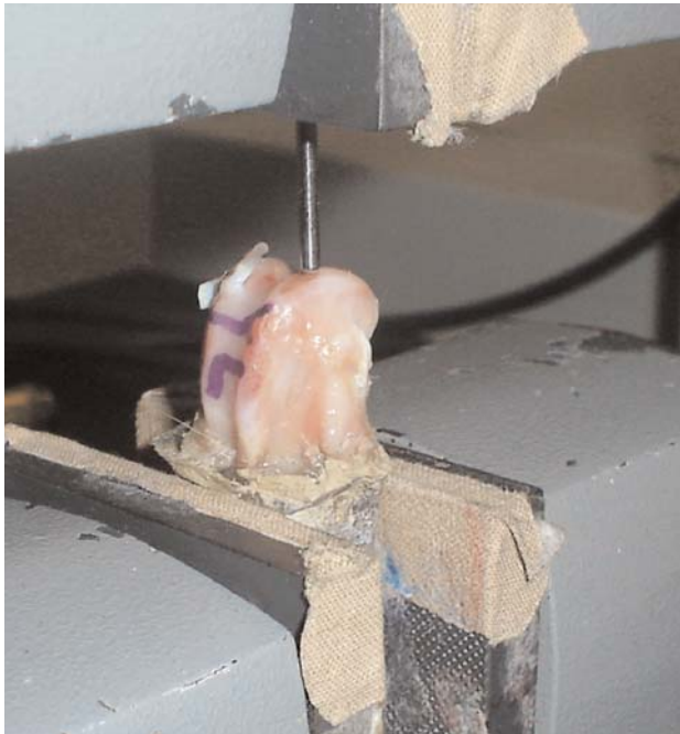
Fig. 2. Assembly of the samples in the indentation testing device. [Color figure can be viewed in the online issue, which is available at www.aott.org.tr ]
