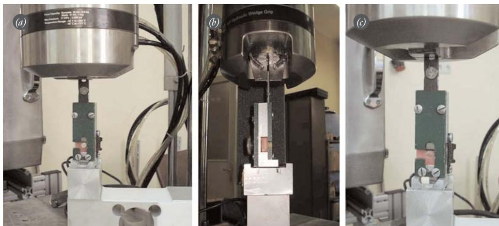
**Fig. 4.** (a-c) Figures show the shearing of PMMA sample in shear test. [Color figure can be viewed in the online issue, which is available at [www.aott.org.tr](http://www.aott.org.tr)]
