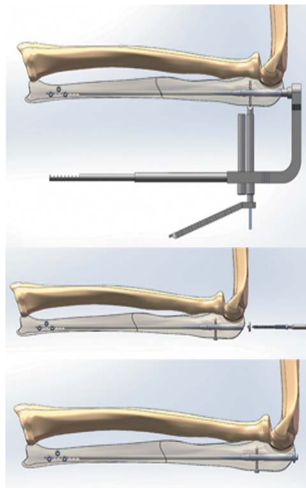
Fig. 7. The proximal end of the ulna nail allows static or dynamic locking. With the oval hole, transverse lateromedial or posteroanterior locking can be done. If necessary, dynamic locking can be done for the compression of the fracture line. [Color figure can be viewed in the online issue, which is available at www.aott.org.tr ]
