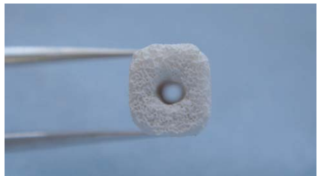
Fig. 2. Tunnel with a 2 mm diameter inside hydroxyapatite ceramic bloc.
