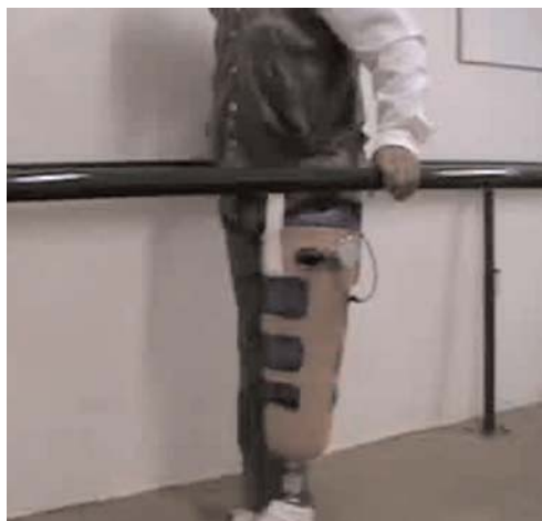
Fig. 2. Application of pneumatic prosthesis for a TF amputee. [Color figure can be viewed in the online issue, which is available at www.aott.org.tr ]
