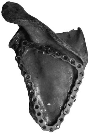
Fig. 5. The new extended anatomical frame plates for the left scapula.
